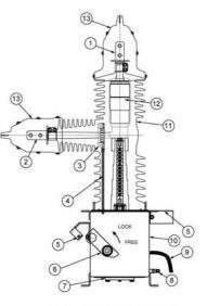
Cross section of E series 38 kV switchgear
