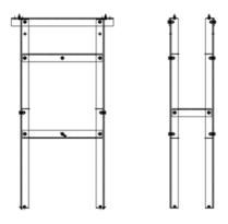
27 kV /38 kV Substation mounting bracket
