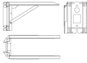
27 kV/38 kV mounting bracket for wooden pole (through holes mounting) (Same mounting bracket for end and center mounting)
