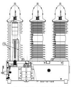
Typical front view of E series 27 kV/38 kV switchgear
