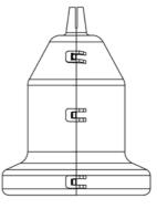
27 kV/38 kV Bird guard (I Side)
