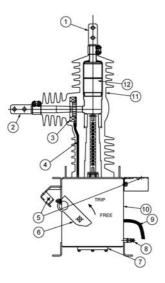
Cross section of E series 27 kV switchgear
