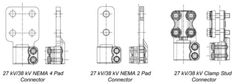
Either one of the above three connectors are required in 6 quantity or recloser.
