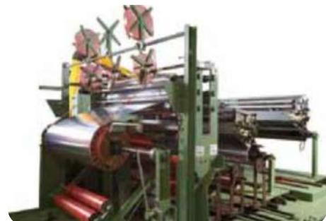
■ Sheet Winding Machine for Low Voltage Coils
