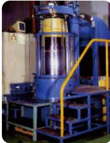
■ Autometed Winding Machine for High Voltage Coils
